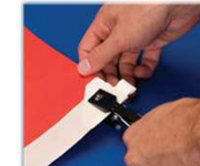
Punch hole with Power Punch
